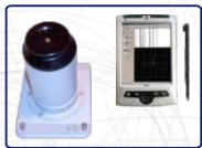
Combination of Viscosity meter BalVis with Pocket PC.
